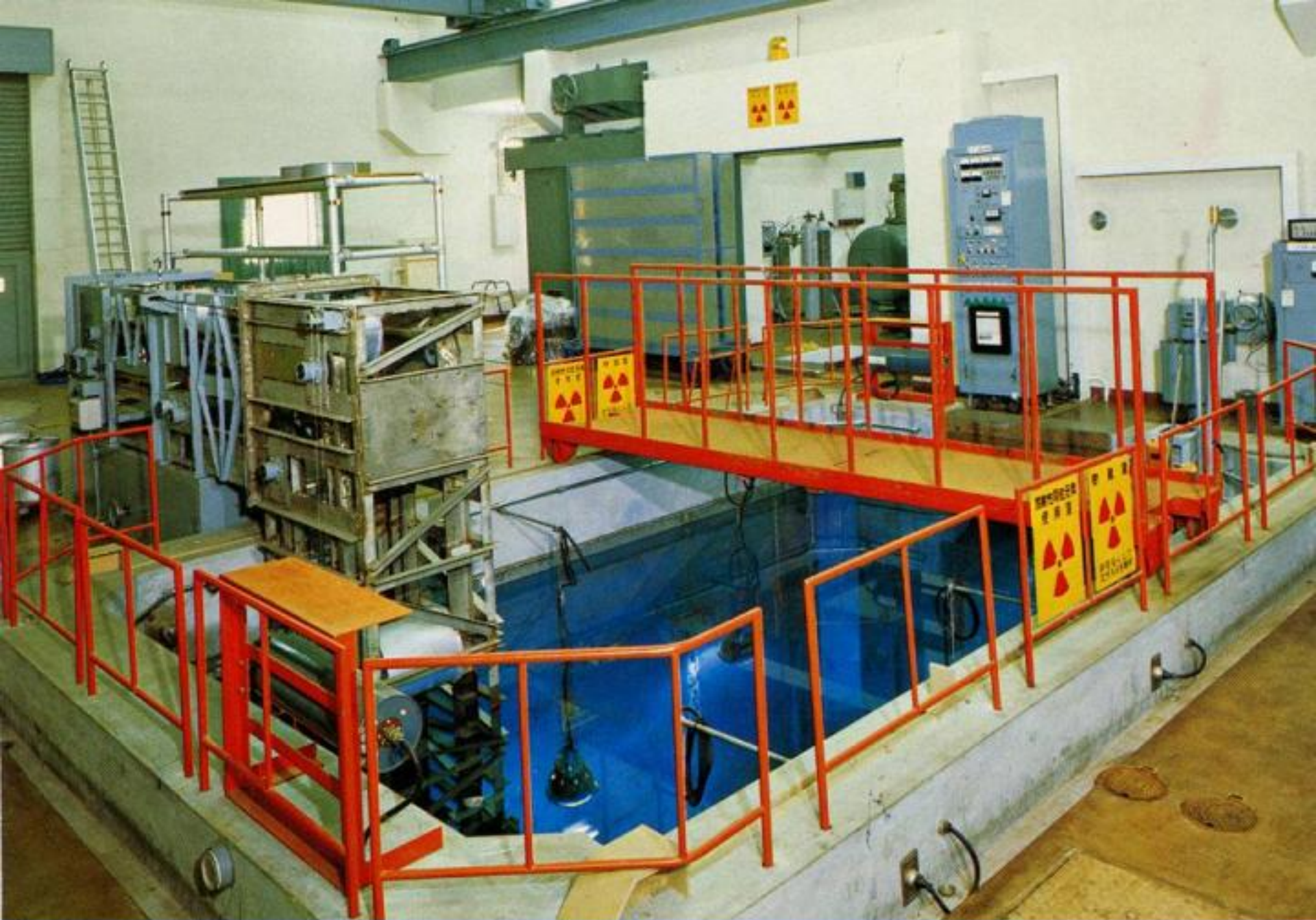
Water pool for ^{60}\text{Co} \gamma -ray sources
