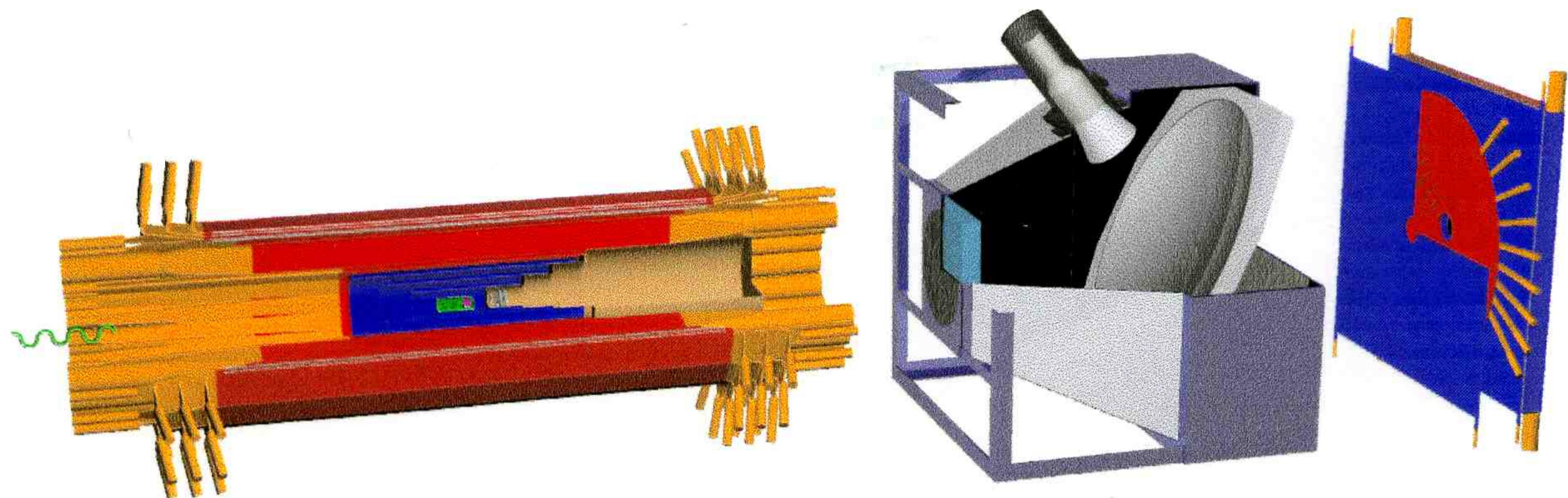
DAPHNE: Three wire chambers and sectorized annulus of plastic scintillators
