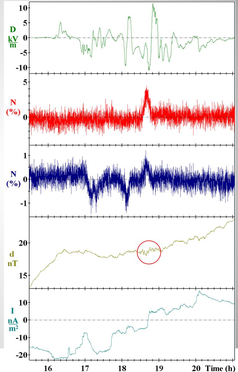
Event on October 15, 2007: complex variation of muons repeats the behavior of h-component of geomagnetic field (daily wave subtracted) with a time delay of 9 min
