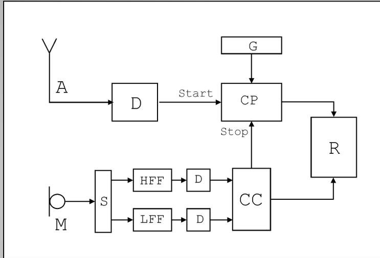
**A** is antenna, **M** is microphone, **D** is discriminator, **S** is splitter, **HFF** and **LFF** are high and low-frequency filters, respectively, **CC** is coincidence circuit, **G** is generator, **CP** is counter of pulses, and **R** is recording device.
