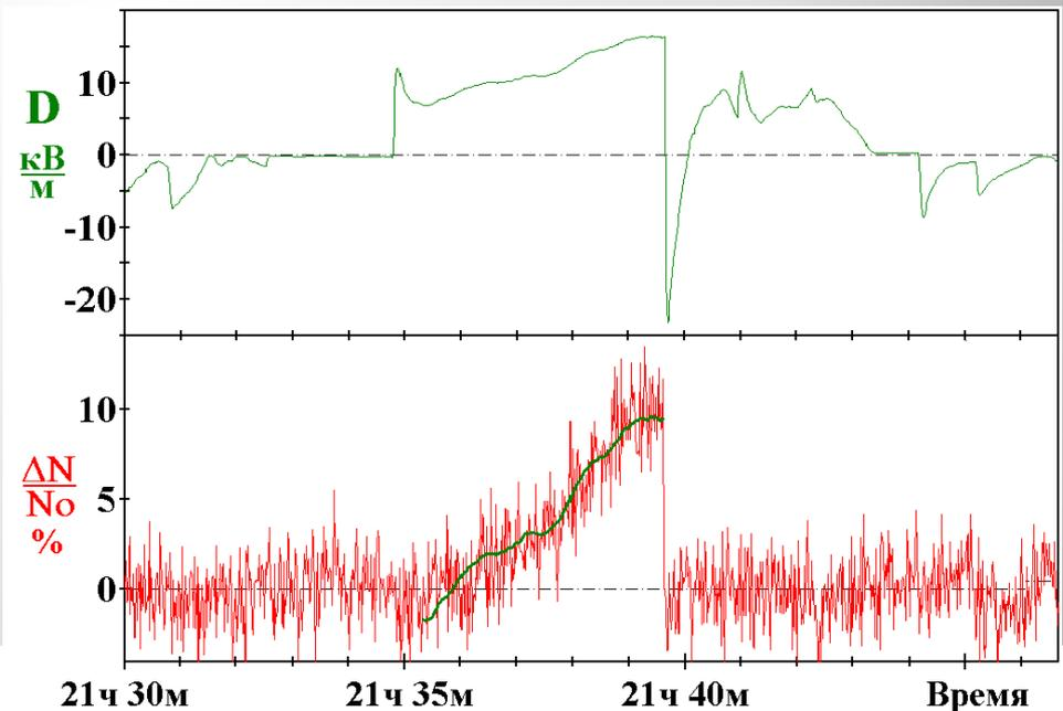
An example of separating independent variations of the hard and soft components during thunderstorm on September 24, 2000
