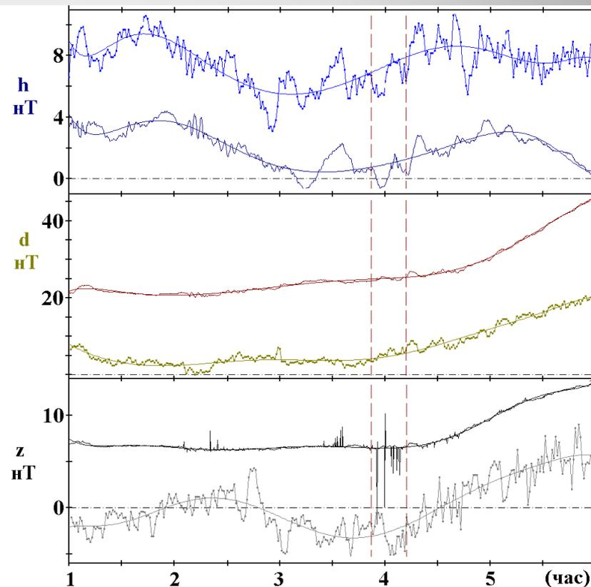
Joint plots of deviations of the magnetic field components from their trends for two stations. Red digits are the numbers of local soft component enhancements that correspond to disturbances of the geomagnetic field measured at the same time in Moscow. Maxima of negative disturbances of the hard component are enumerated by blue digits.
