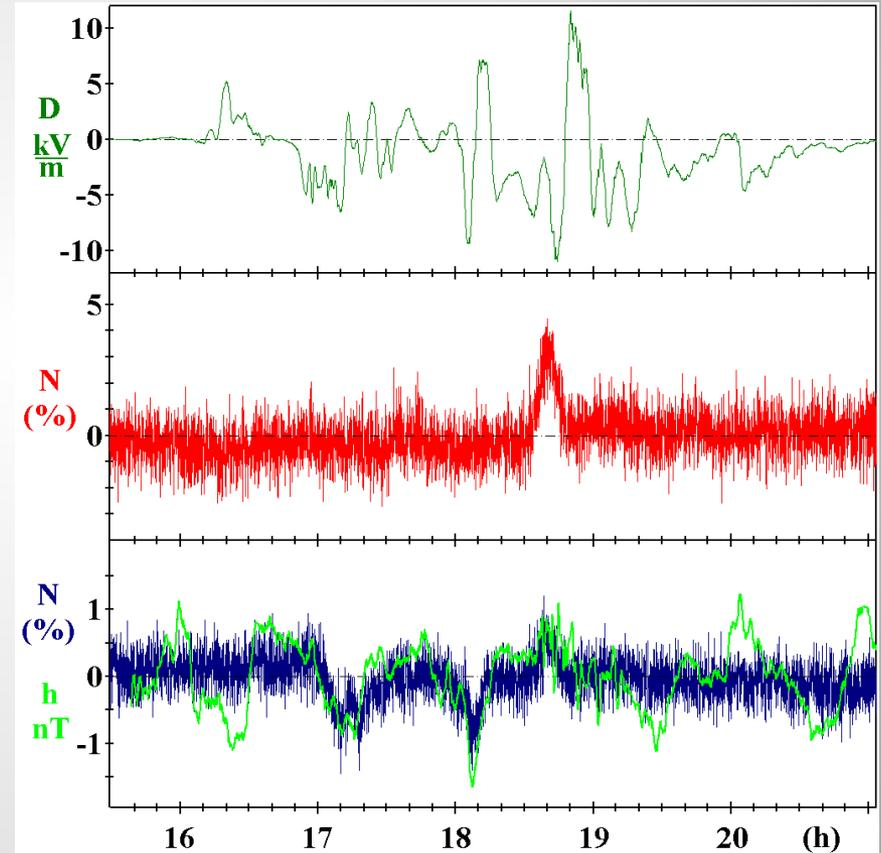
Variations of three components of the geomagnetic field on July 31 and August 1, 2008 according to stations Baksan and Moscow. Interval of averaging is 15 s.
