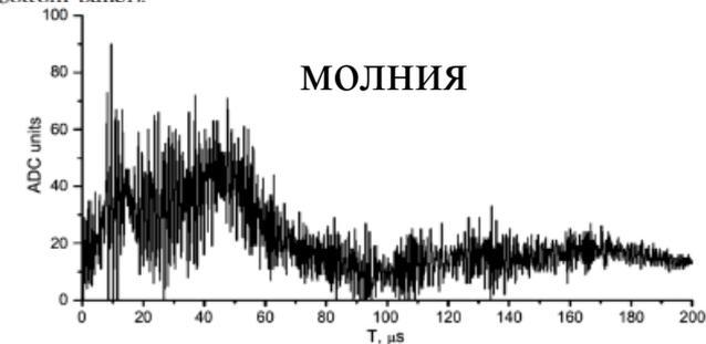
FIG. 3. Noise pulse shape produced by lightning.
