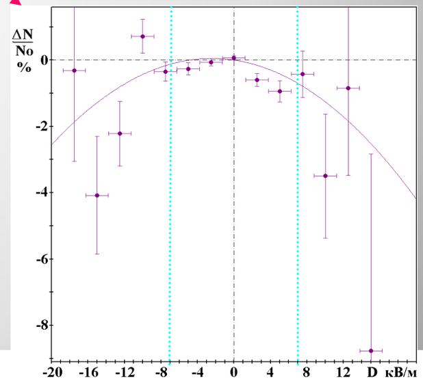
Muons with  $E_\mu > 100 \text{ MeV}$ , deviation from the mean intensity as a function of near-ground electric field strength (weighted average curve, summation over separate thunderstorms)
