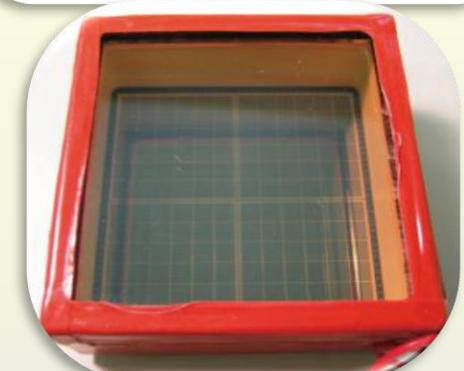
420 HAPD (Hybrid Avalanche Photo Detector QE = 28% at 400 nm, gain ~ 10<sup>5</sup>) modules in 7 rings
