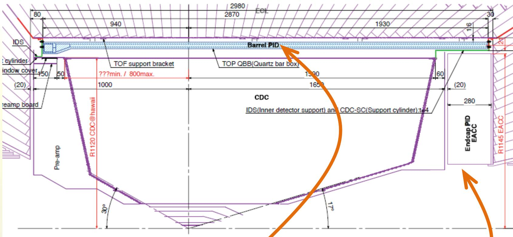
Two dedicated particle ID devices: both RICHes → designed to fit into available space
