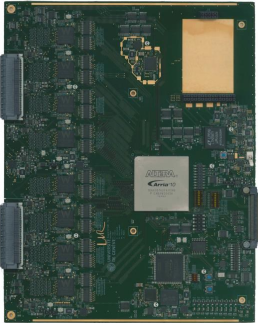
Front-End Board (14 boards per crate) – analog processing, ADC, bias voltage to the MPPCs & CITIROC chips per board – 256 channels
