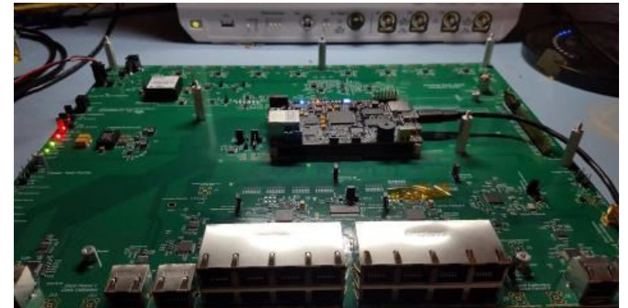
Master Clock Board – external to magnet, hardware connections to the beam triggers
