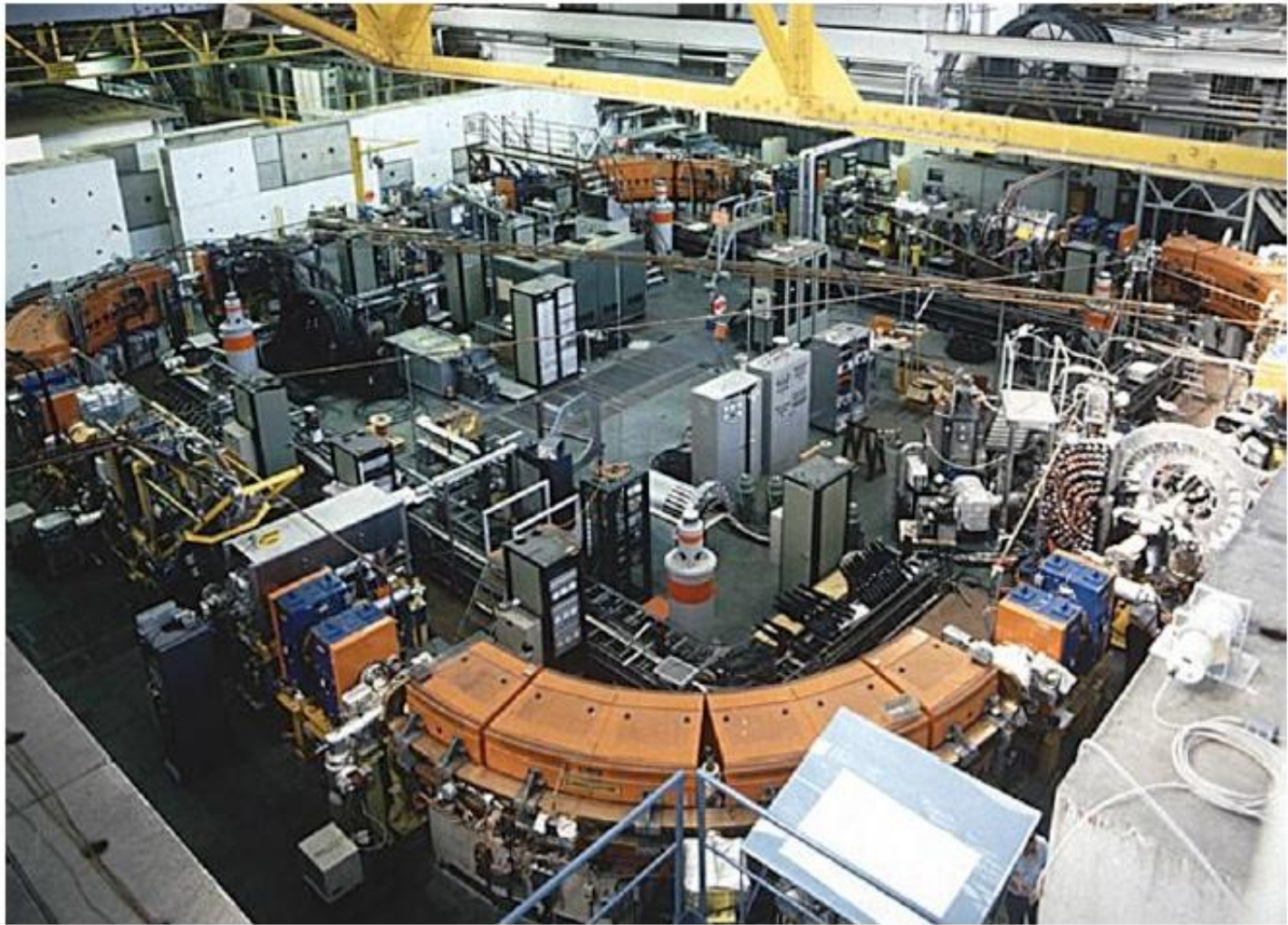
Fig 1. Stochastic Cooling at LEAR (CERN). Different signal transmission lines cutting through the ring can be seen (CERN photo 9007366)
