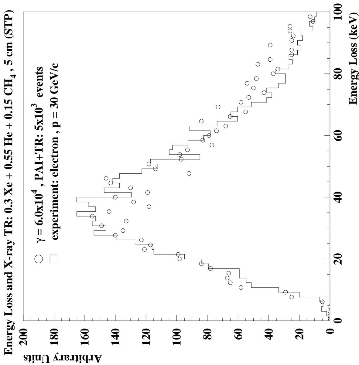
**Fig. 4.** The total energy loss distribution produced by electrons with a momentum of 30 GeV/c in a gas mixture 0.35Xe + 0.55He + 0.15CH<sub>4</sub>, 5 cm thick at 1 atm. The histogram is the experiment [15], open circles are GEANT4 simulation. XTR radiator:  $350 \cdot (\text{CH}_2/\text{CO}_2 = 0.019/0.6)$  mm.
