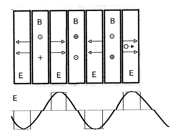
The proper cavity frequency  $\omega_c$  and the time of light  $\tau$  are matched for  $\omega_c \tau = \pi/2$ . For smaller  $\omega_c$  the wavelength is larger to keep the synchronism.
