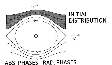
Due to radiation reaction ultralight particles bunch in the decelerating field providing coherent radiation. This process comes to saturation
