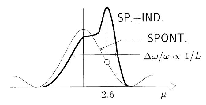
The linewidth of sp. radiation is determined, at least, by the limited interaction length L. The preferential mode with  $\mu=2.6$  grows exponentially causing narrowing of the spectral line (lasing).
