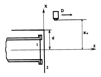
Experimental setup is shown in the fig. The source of the relativistic electron was microtron. Accelerated electrons had energy og 7.4 Mev. Then the bunch passed through interspace of length 1.5m and was extracted through the foil of thickness 100  $\mu$ m. The detector D could be positioned at various distances from the beam axis z and moved parallel to this axis.
