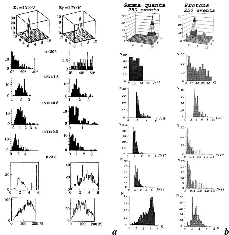
Fig. 1 a - Monte Carlo distribution of image parameters for gamma-quanta and proton showers of 1 TeV and b - experimental SHALON distribution of image parameters for gamma-quanta and proton showers with energy more than 0.8 TeV.
