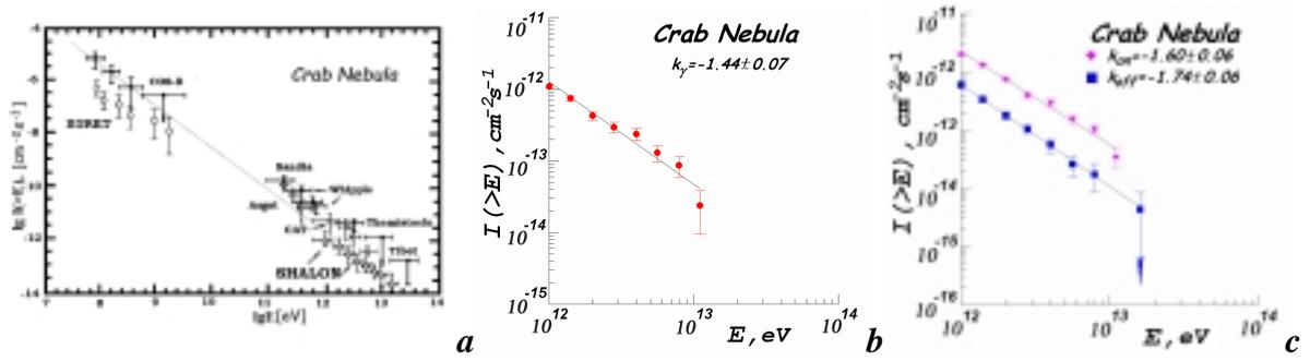
Fig. 1 a - The Crab Nebula gamma-quanta integral spectrum by SHALON in comparison with other experiments; b - the Crab Nebula spectrum  $dF/dE \sim E^{-2.44 \pm 0.07}$ ; c - the spectrum of events from Crab Nebula, including 10-15% contribution of background events  $dF/dE \sim E^{-2.6 \pm 0.06}$ , the spectrum of background events observed simultaneously with source  $dF/dE \sim E^{-2.74 \pm 0.06}$ .
