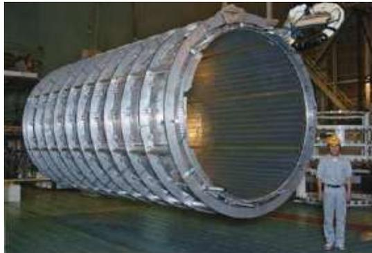
Figure 6. Bare central solenoid in the factory after completion of the coil winding.
