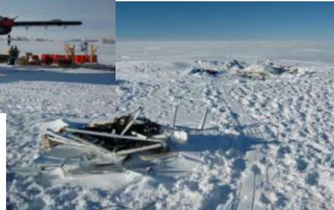
ATIC is designed to be disassembled in the field and recovered with Twin Otters. Two recovery flights are necessary to return all the ATIC components. Pictures show recovery flight of ATIC-4
