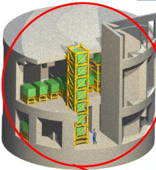
On-Axis Neutrino Monitor (INGRID) Monitor: \nu beam direction
