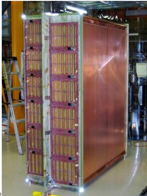
Micromegas readout plane
