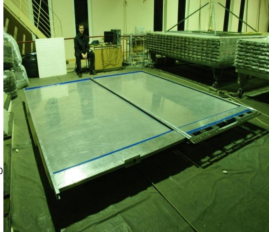
Scintillation detectors developed in Mephi
