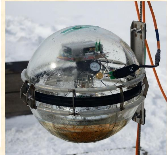
D=10 inch. SBA photocathode QE  $\approx 35\%$  @ 400nm; Gain  $\sim 10^7$ , dark count  $\sim 8$  kHz
