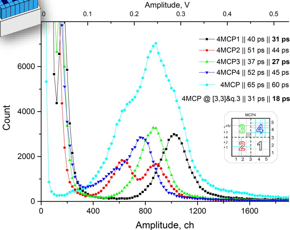
Results for the **repaired NBI MCP** with different combinations of fragmented radiators.
