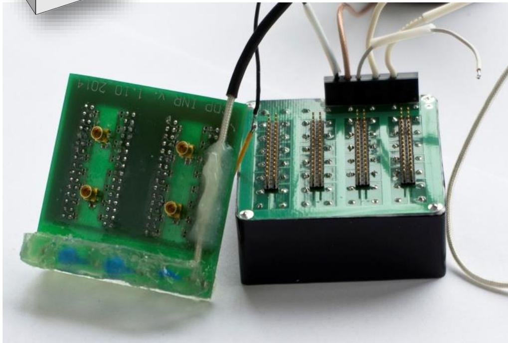
**Modified** variant has RF grounded MCP out electrode, reduced anode-ground capacitance, and equalized propagation time from individual anodes to the output connectors.
