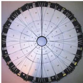
**V0 & T0** Provide triggers, luminosity monitoring, background reduction, collision time (for PID), centrality, and event plane determinations
