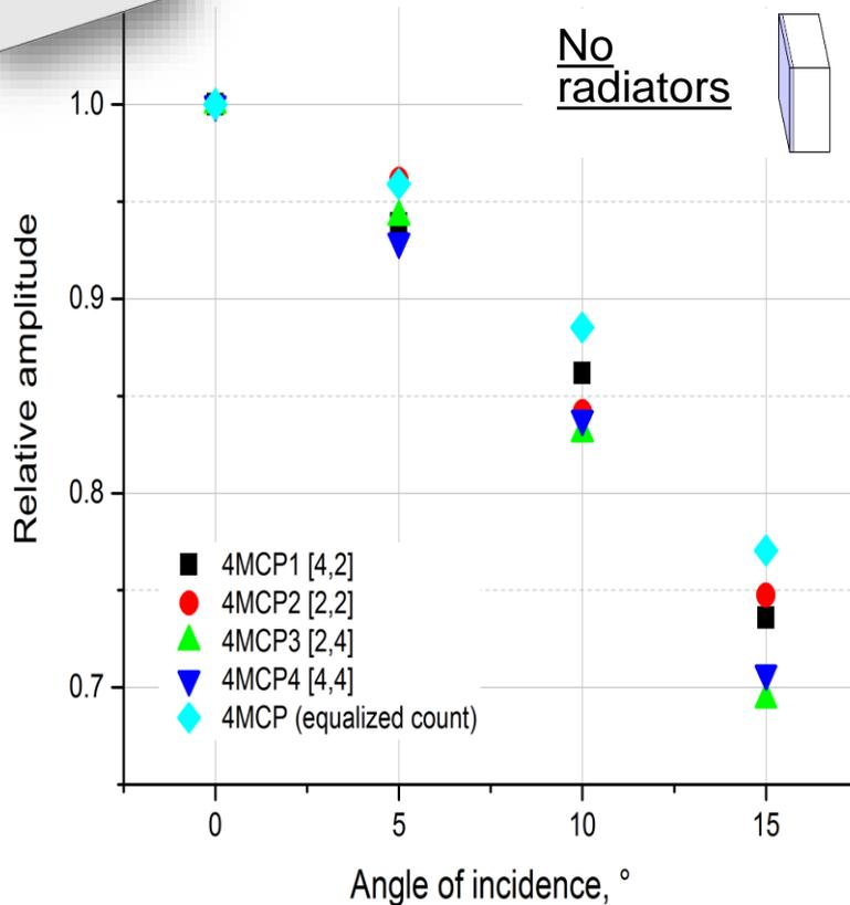
If T0+ at side C is flat, particles would hit the radiators under the corners of up to **12.6°**.
