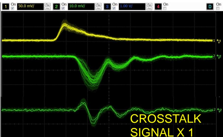
The leading edge is unstable, depends on charge distribution between individual anodes of the three illuminated quadrants. Oscillation on the trailing edge can be seen. The crosstalk signal is large.
