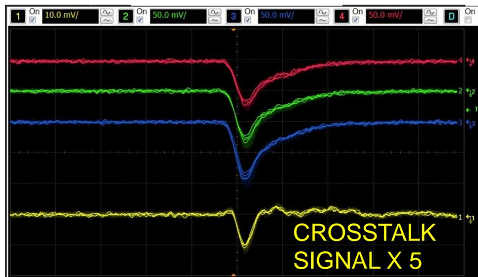
Signals from the 3 illuminated quadrants are stable and without oscillations. The crosstalk signal (on the darkened quadrant) is now  $\sim 5x$  smaller and has only a negative component. There is no time shift. The trailing edge is  $1.5x$  shorter.
