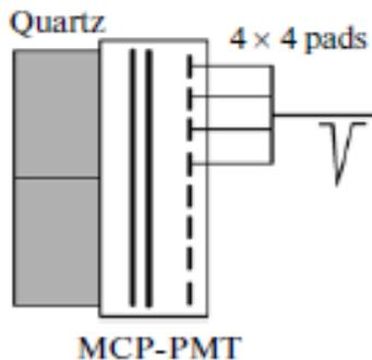
**MCP-PMT** : The MCP-PMT **XP85012** with 64 anode pads is transformed into the 4channel photo detector by merging 16 pads ( $4 \times 4$ ) of each cell into a single channel
