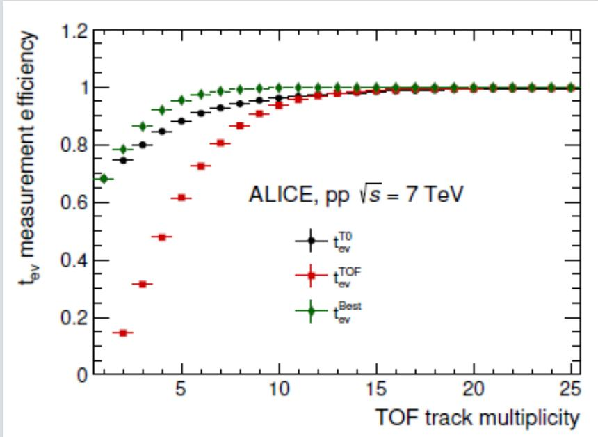
In pp collisions, for very low multiplicity events, the current T0 detector can provide a  $t_{ev}$  measurement with an efficiency of the order of 70% that increases with the track multiplicity. At the same time, for all events having high multiplicity, the  $t_{ev}^{TOF}$  method is able to provide a  $t_{ev}$  measurement.
